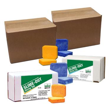
**DIRECTIONS FOR USE:** One Slime-Out can last for an entire normal cooling season. Use One Slime-Out yellow tab for (each 7 tons or less), or Blue Tab for (each 20 tons or less) of air conditioning. Place One Slime-Away in the condensate pan and position so that the condensing moisture drips on or runs over the Slime-Out tab. The dissolving action forms a gel and locks the Slime-Out into place, slowly releasing treatment for extended cleaning action.
